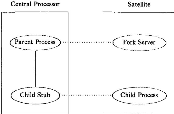
**Figure 13.5.** Fork on the Central Processor
