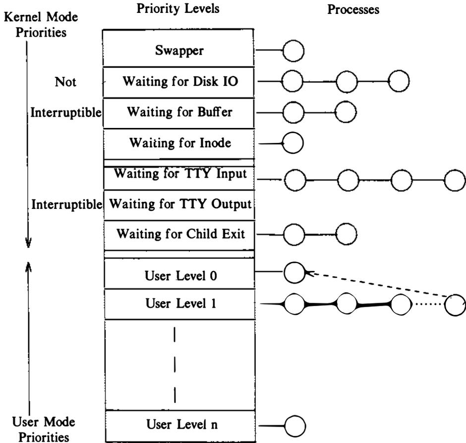
Figure 8.3. Movement of a Process on Priority Queues
