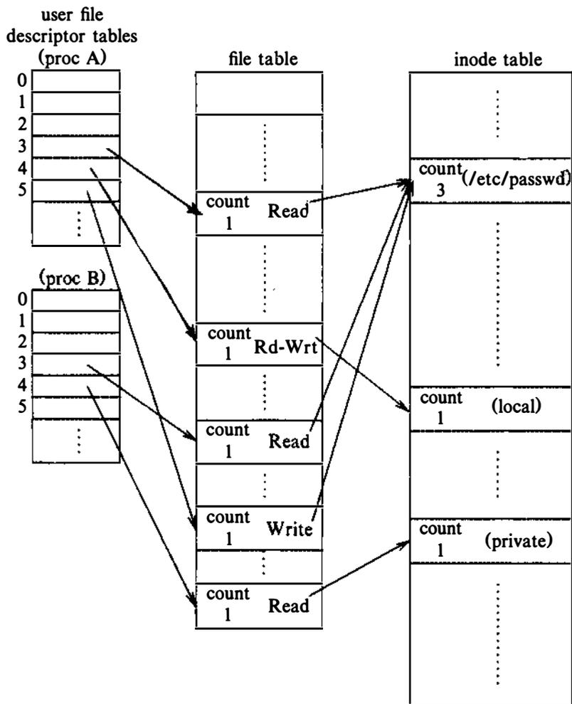
Figure 5.4. Data Structures after Two Processes Open Files
