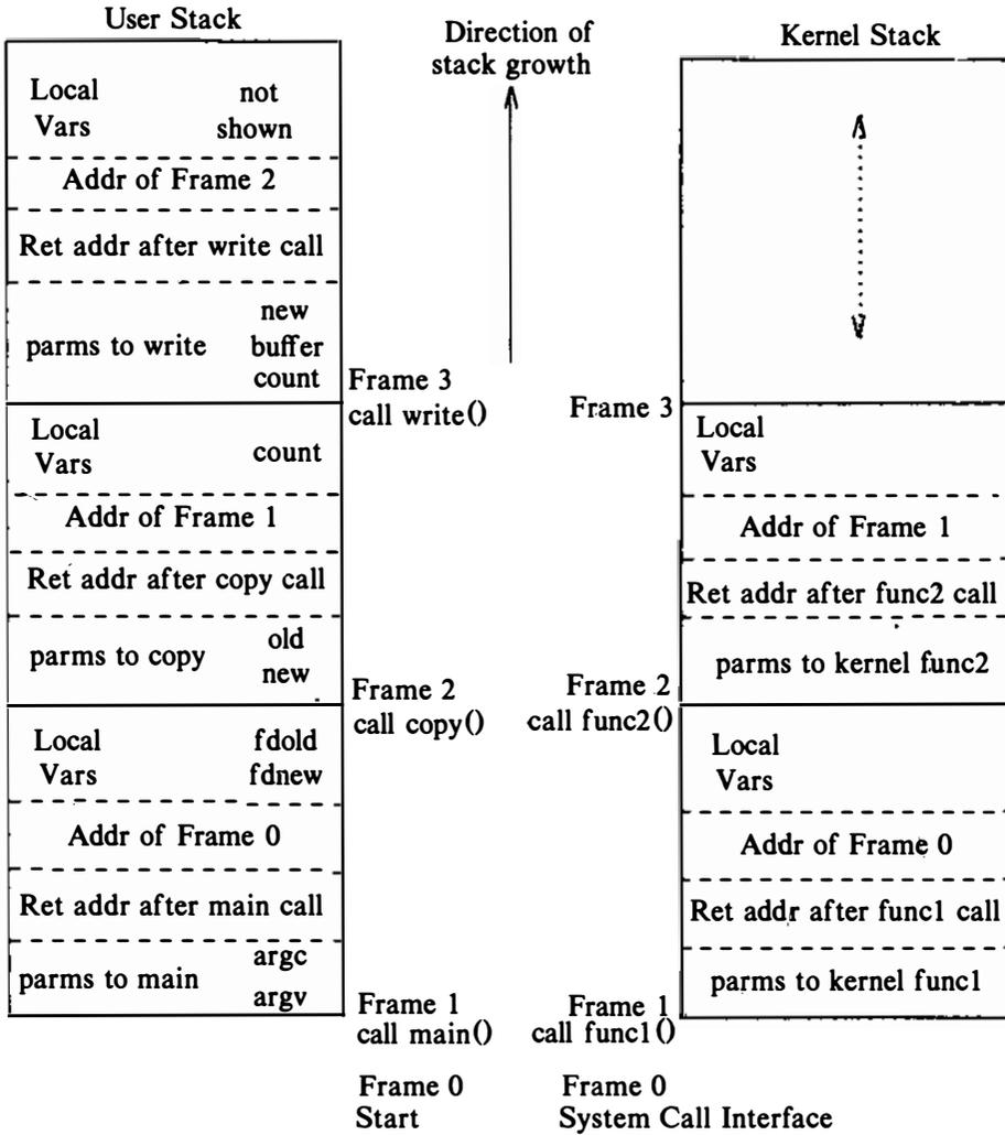
Figure 2.4. User and Kernel Stack for Copy Program
