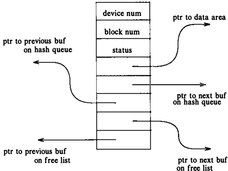
Figure 3.1. Buffer Header
