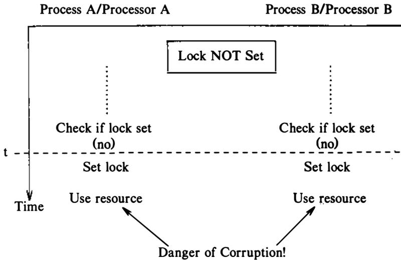
**Figure 12.5.** Race Conditions in Sleep-Locks on Multiprocessors
