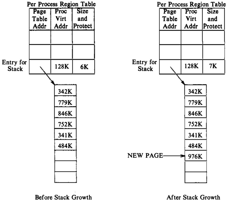
Figure 6.22. Growing the Stack Region by 1K Bytes
