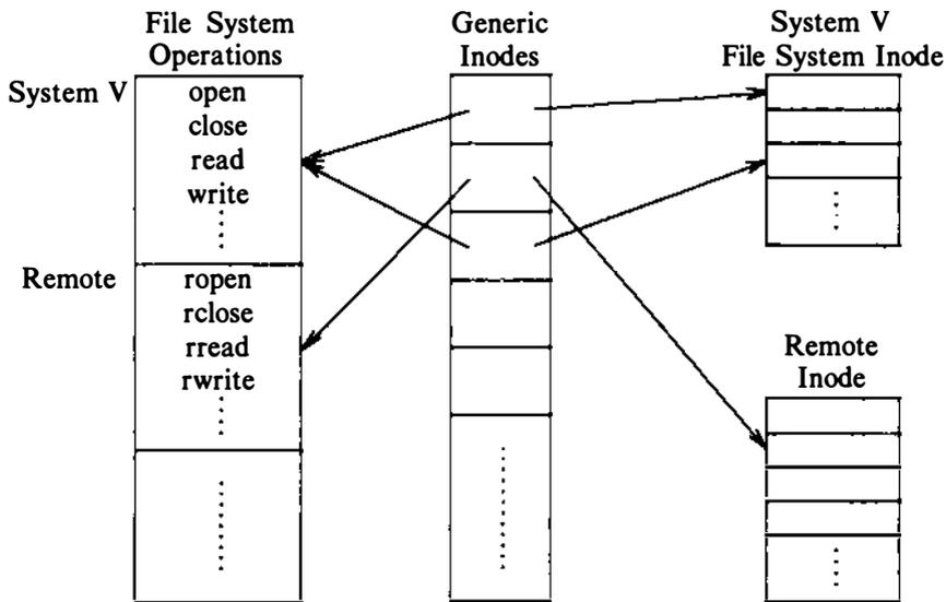
**Figure 5.34.** Inodes for File System Types
