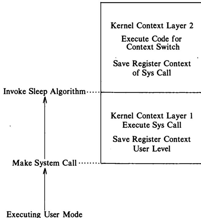
**Figure 6.29.** Typical Context Layers of a Sleeping Process
