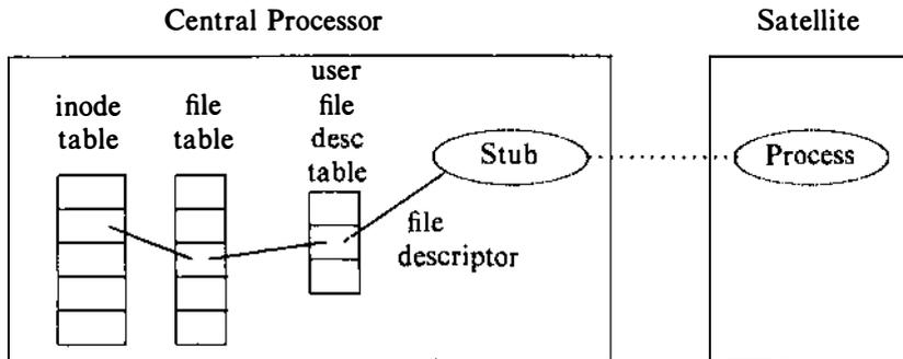
Figure 13.4. Open Call from a Satellite Process
