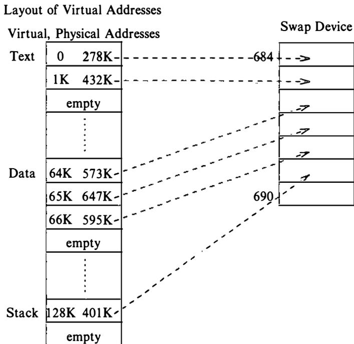
Figure 9.6. Mapping Process Space onto the Swap Device
