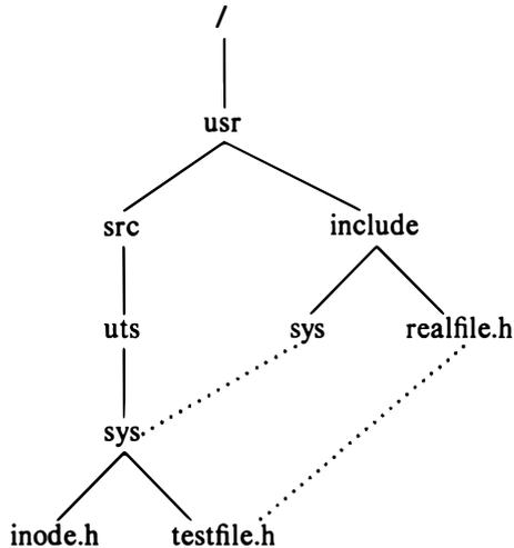
Figure 5.28. Linked Files in File System Tree
