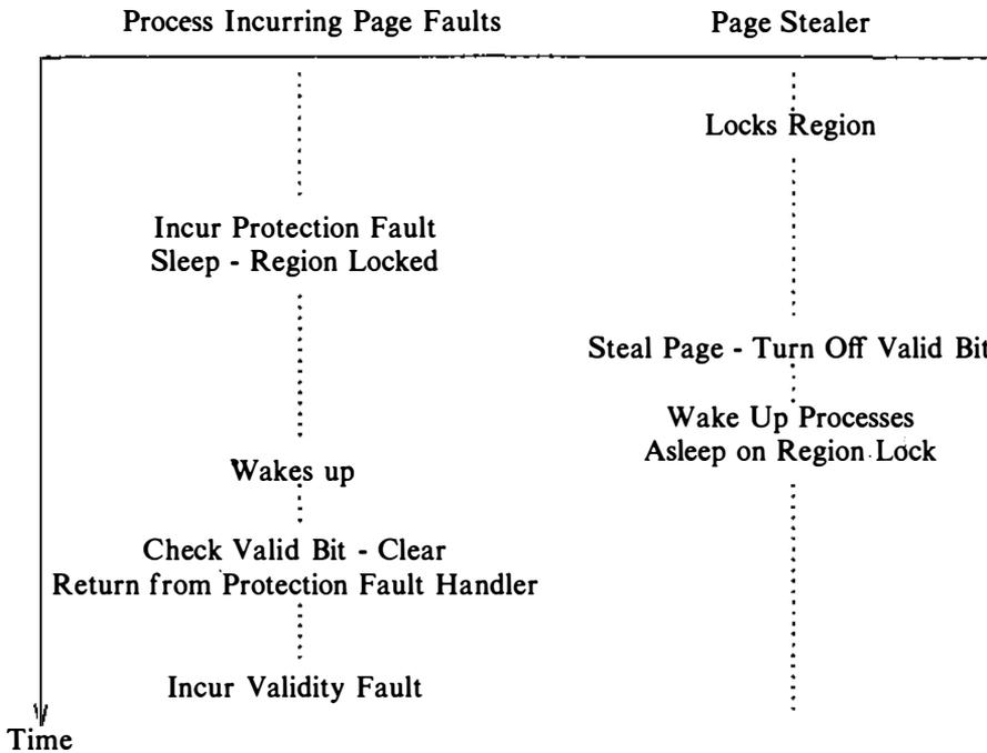
Figure 9.27. Interaction of Protection Fault and Validity Fault
