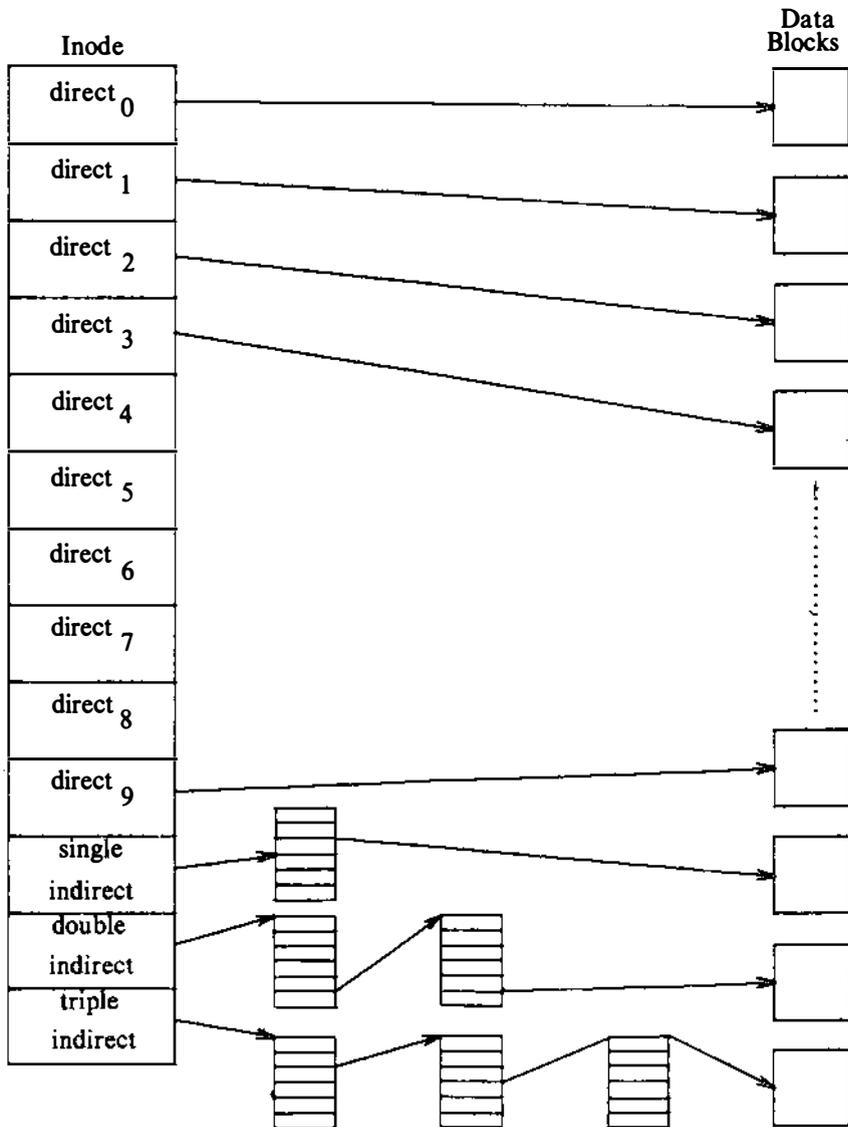
Figure 4.6. Direct and Indirect Blocks in Inode
