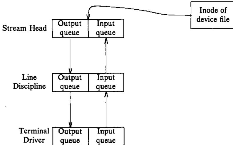
**Figure 10.22.** Pushing a Module onto a Stream
