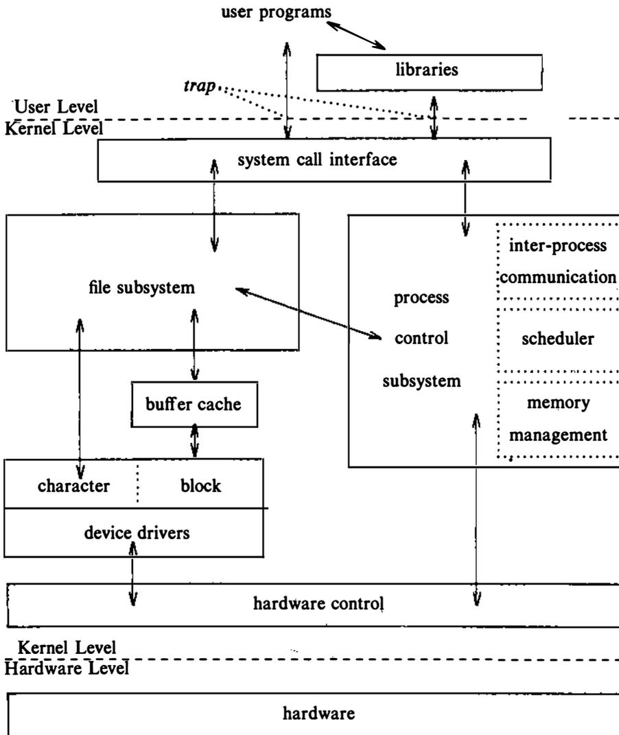
**Figure 2.1.** Block Diagram of the System Kernel
