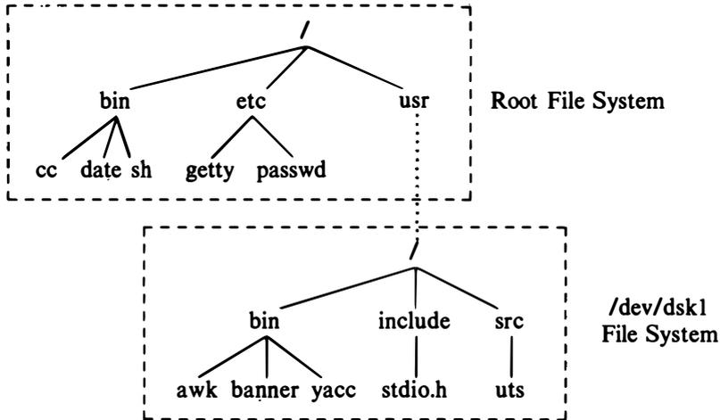
**Figure 5.22.** File System Tree Before and After Mount
