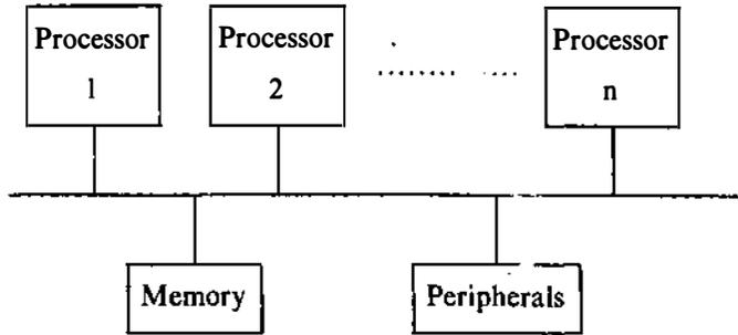
Figure 12.1. Multiprocessor Configuration
