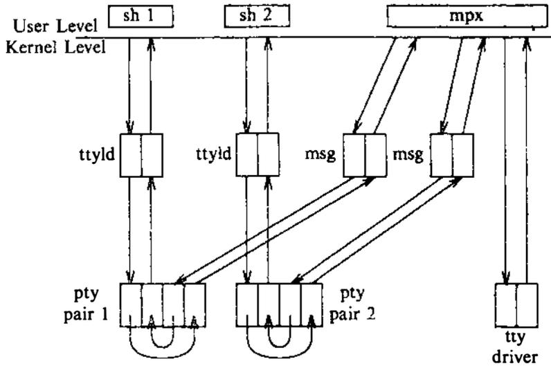
Figure 10.23. Windowing Virtual Terminals on a Physical Terminal
