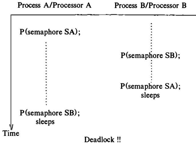
**Figure 12.11.** Deadlock because of Reversed Order of Locking
