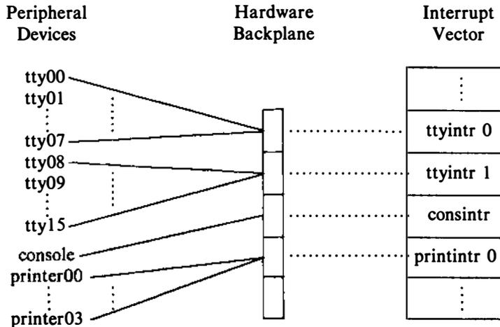
Figure 10.6. Device Interrupts
