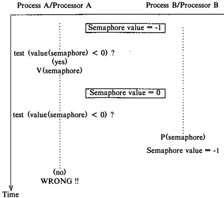
Figure 12.10. Failed Simulation of Wakeup with V
