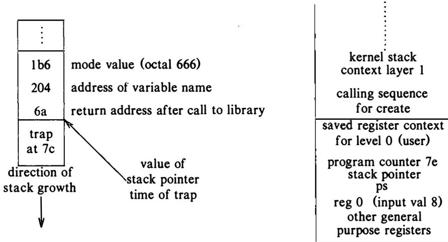
Figure 6.14. Stack Configuration for `creat` System Call
