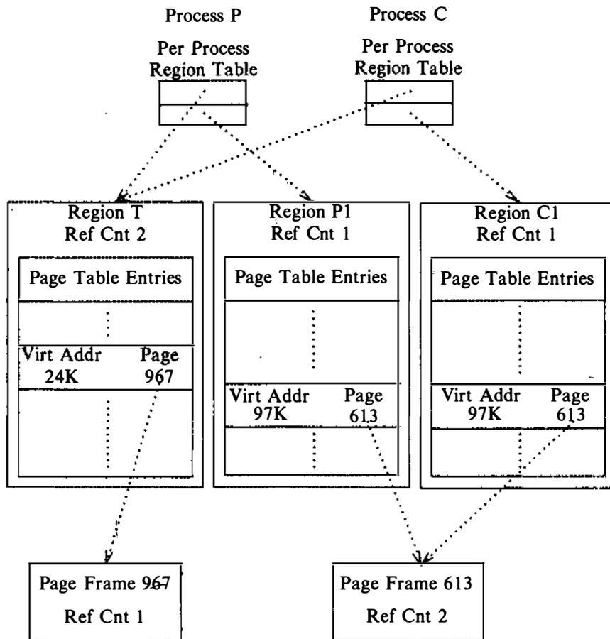
**Figure 9.15.** A Page in a Process that Forks
