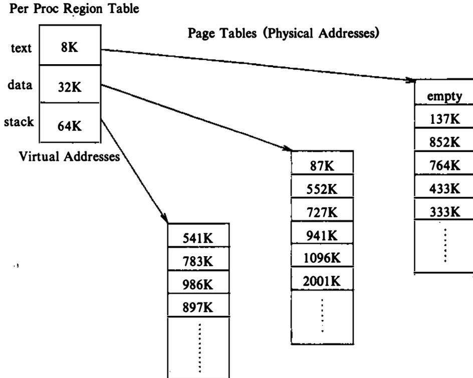
Figure 6.5. Mapping Virtual Addresses to Physical Addresses
