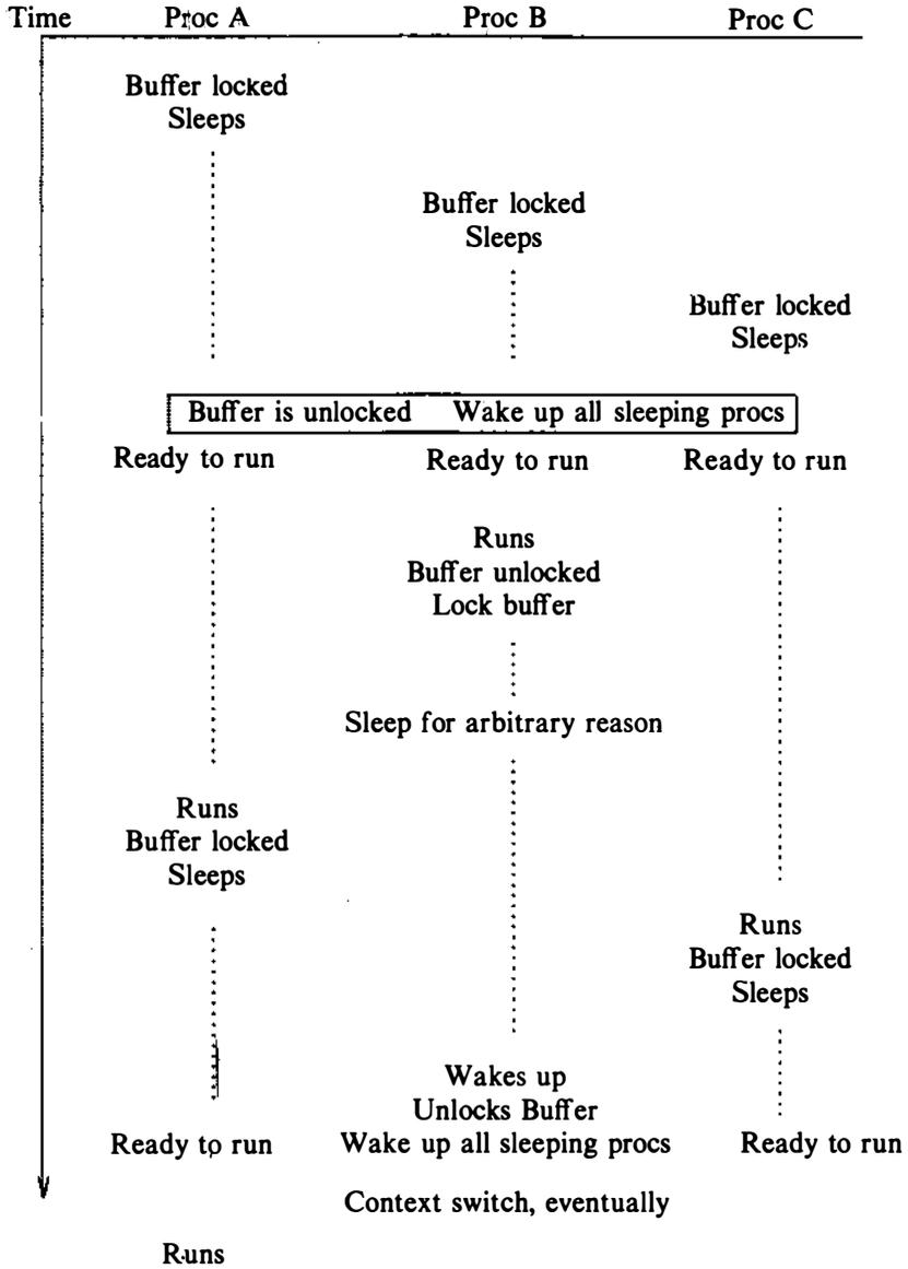
Figure 2.9. Multiple Processes Sleeping on a Lock
