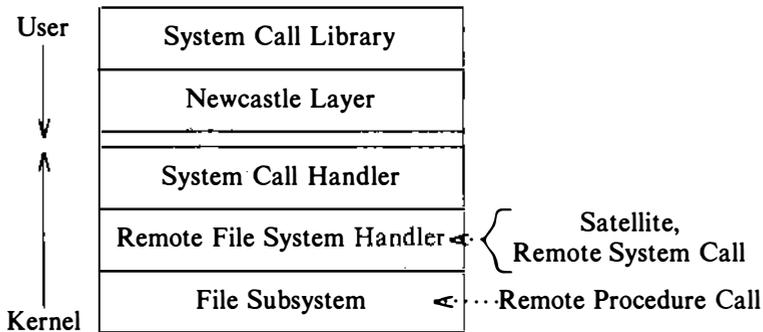
Figure 13.12. Conceptual Kernel Layer for Remote File Access
