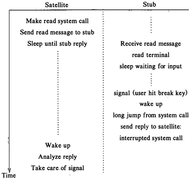
Figure 13.8. Interrupt in Middle of a System Call
