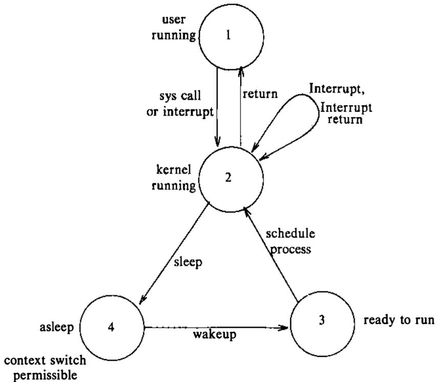
**Figure 2.6.** Process States and Transitions
