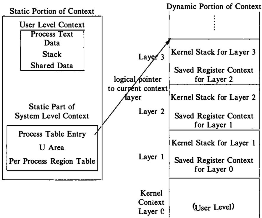
Figure 6.8. Components of the Context of a Process
